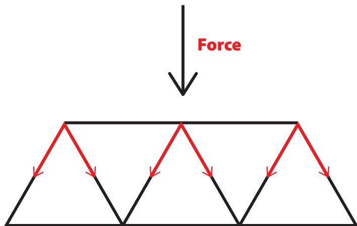
The forces are distributed further and therefore less stress is on each beam!
