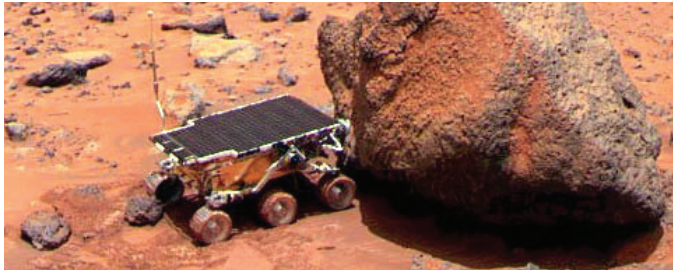
Pathfinder's Sojourner Rover is taking its Alpha Proton X-ray Spectrometer measurement of the Yogi Rock (NASA). This instrument measured the elements in the rock. http://commons.wikimedia.org/wiki/File:Pathfinder01.jpg
