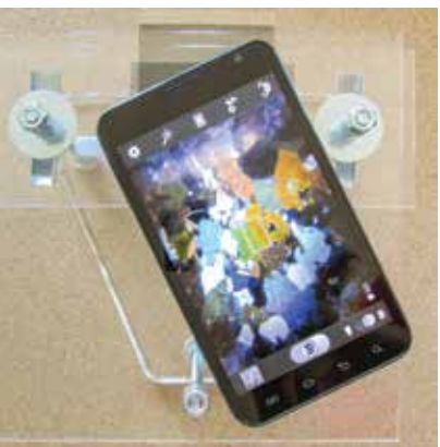
Igneous rock thin section as viewed with Smart Device microscope
